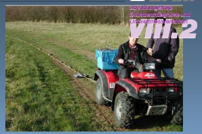
Geoelektrics "pulled array" (IGM/IRIS)
